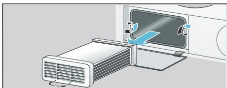
6. Flush water through the heat exchanger from all sides to completely remove all fluff.
