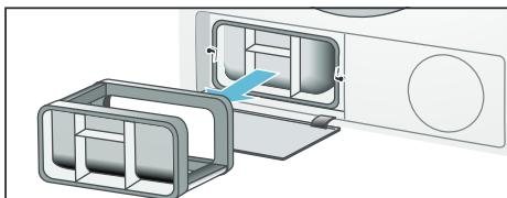
5. Remove the heat exchanger.
