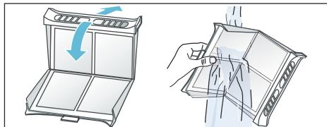
6. Dry the fluff filter, close it and reinsert the fluff filter.
