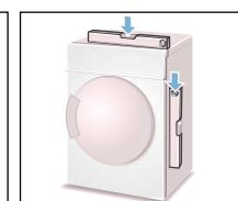
Incorrect alignment may cause high noise levels, vibrations and improper movement of the drum.
