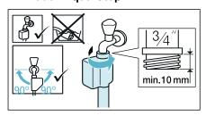
**Tip:** Connect also an external water filter (depending on the model) between water supply hose and tap. The filter filters dirt particles out of the water.
