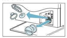
Refit and screw on the pump cover. The handle must be in a vertical position.
