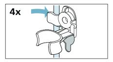
b) Insert and tighten the screws.
