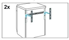
**3.** Undo and remove the screws on the horizontal transport strut.
