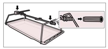
3. Slide the universal pan into shelf position 1 and slide the rotary spit into the motor mount.
