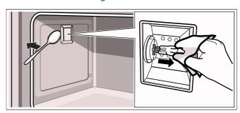
7. Replace the oven light bulb with a bulb of the same type:
