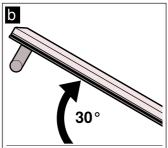
4. Raise the oven door slightly and pull it out. Note: Do not fully close the oven door. The hinges could become bent and the enamel could be damaged.
