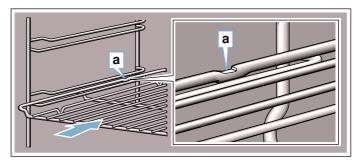
When inserting baking trays, ensure that lug **a** is at the rear and is facing downwards. The sloping edge of the accessory **b** must be facing towards the appliance door.
