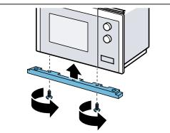
6. Secure the four supporting feet to the base of the microwave.
