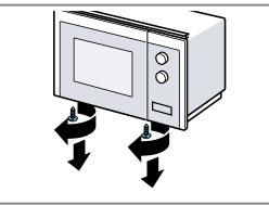
5. Secure the built-in frame on the microwave base with the two outer screws.
